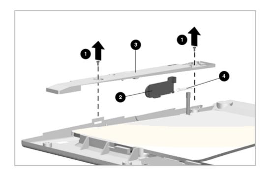
Figure 5-42. Removing the Battery Release Assembly
